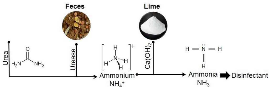
**Figure 2. Chemical reaction for Safe Sludge process (Dr. Temi Ogunyoku).** The two steps take place at different pH values and thus must be separated either temporally or spatially.
