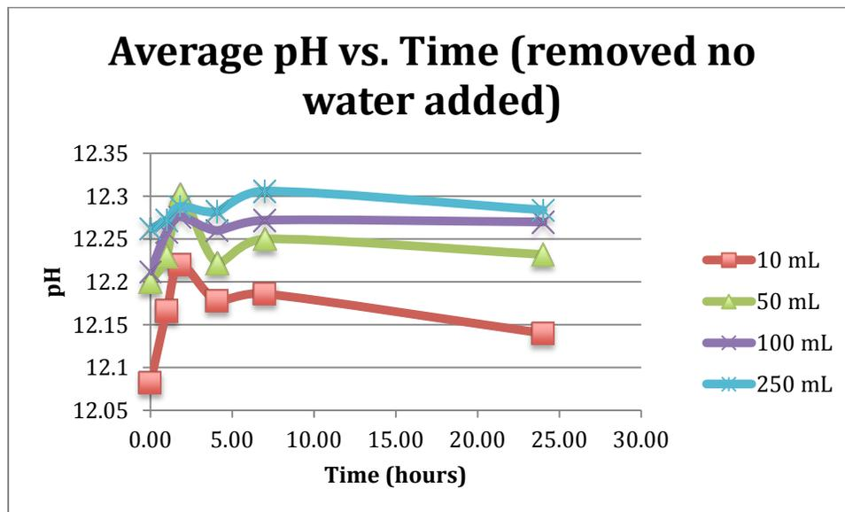
Figure 11. Average pH vs. time for watered samples. All pH measurements were above pH 12. All samples showed a slight decrease in pH from 6 hours to 24 hours.
