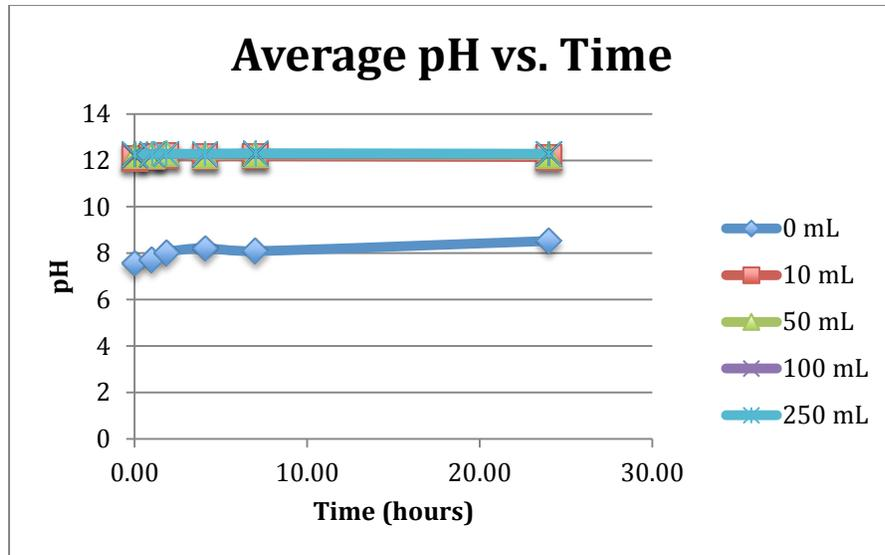
Figure 10. Average pH vs. time for all samples. The no-water sample showed a pH value far below (4 pH units) the other four samples.
