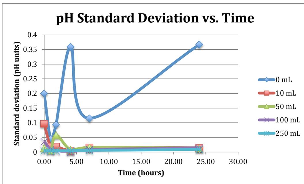
**Figure 12. Standard deviation vs. time where standard deviation is a measure of mixing.** Again the no-water sample is an outlier, but this time with a higher standard deviation than the other four samples.
