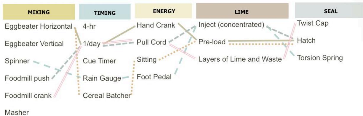
**Figure 5. Matrix of five of six challenge components.** Here mixing, timing, energy (power), lime addition, and sealing are shown. We chose to save cleaning for after our designs were more concrete. Lines connecting elements in different columns show the different prototypes designed (Team Binder 3d).
